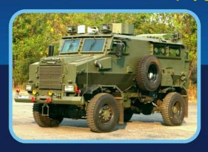
It is an upgraded version of erstwhile Mine protected Vehicle 4×4 which was also produced by Vehicle Factory Jabalpur. Major upgradations and add-ons include Engine power, HVAC, rear view camera, Self recovery winch, rotating searchlights & power operated rear view mirror etc.
