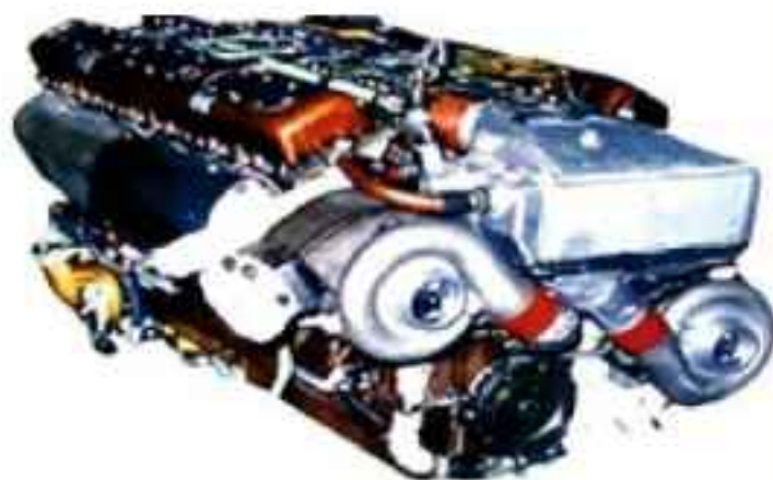
Upgrading of power of T-72 Tank from 780 HP to 1000 HP Engine
